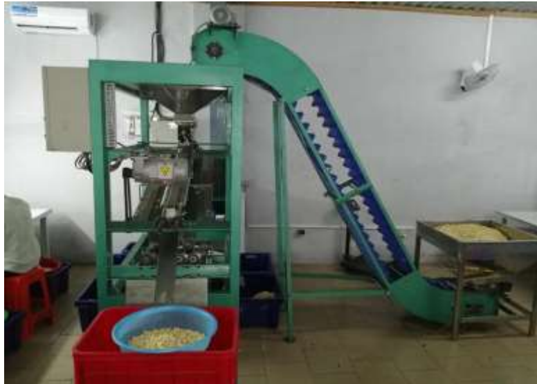
Plate 2.6: Cashew kernel grading machine
