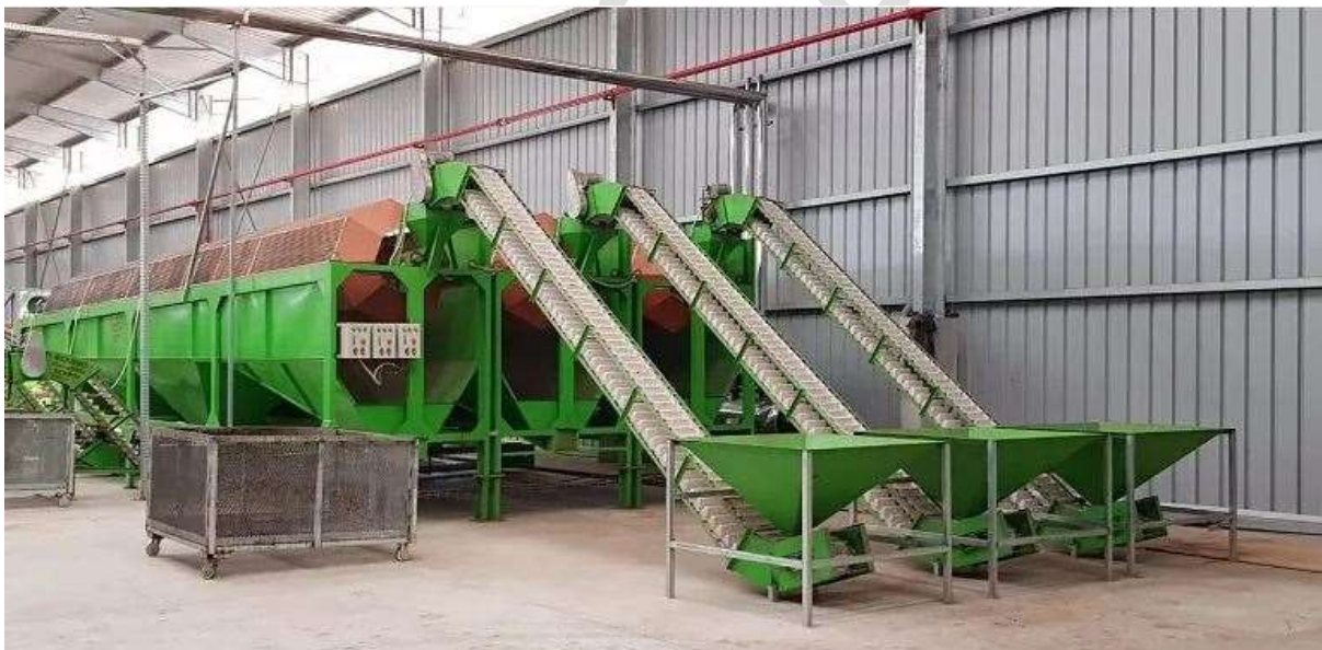
Plate 3.1: Raw cashew nut cleaning and calibration machine Source: DAI, 2022
